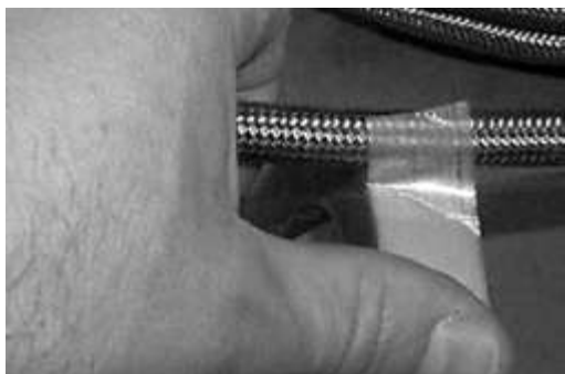
Tape hose before cutting.
